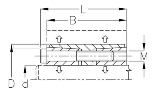
B mm = 54d H8 mm = 38D mm = 75Fit tolerance = Aksel h8, Nav H8
